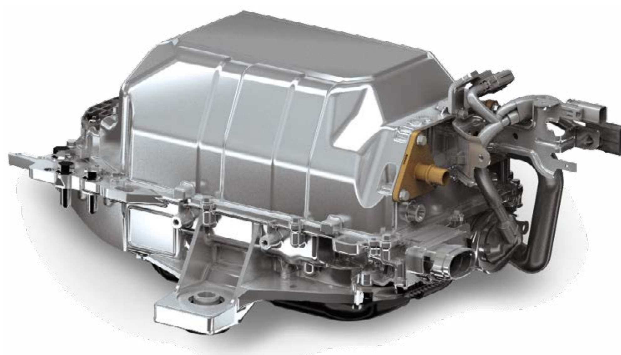
Fuel cell boost converter
